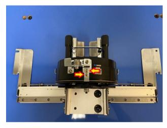
3. Loosen the two screws (illustrated above) place the small metal tab (or star washer) between the cable and silver bar so that the bar pinches the cable.
