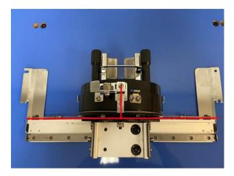
a. Tip: Loosen the two screws (illustrated below) to allow you to move the cap driver left and right in order to get it centered. You can do this by pushing on the black drum from one side to force it to slide on the cable (not rotate).
