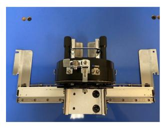
2. Position the cap driver so the bottom lever is up on top and in the middle of the cable. You can measure this to make sure it is dead center in the cap driver.
