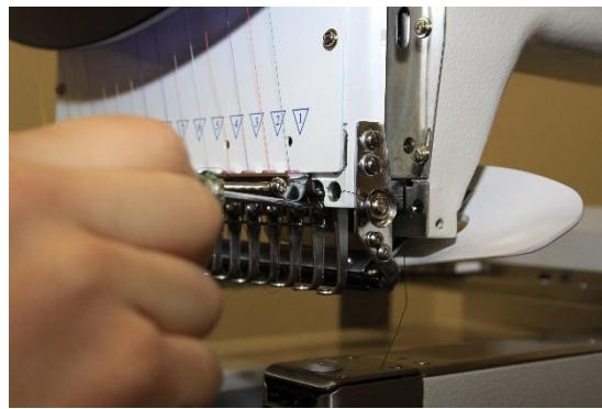
5. Place the needle alignment tool on the face of your needle. If it points to the right or to the left, loosen the needle clamp screw slightly and adjust the needle so that the eye of the needle is straight ahead. Your needle alignment tool will then point straight ahead as well.
