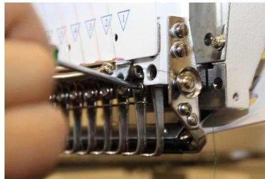
2. Using your needle nose pliers, remove the old needle
