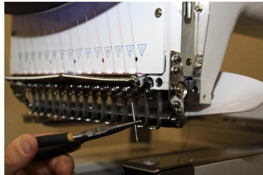
3. Using your needle nose pliers, insert the new needle so that the scarf is pointed towards the back of the machine
