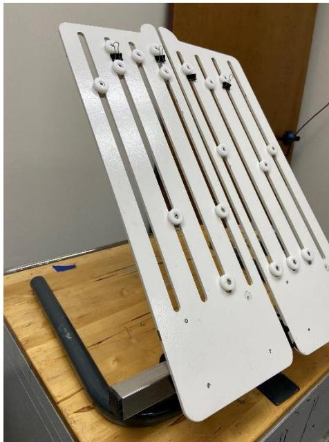
4. To set it up for production, you can move the white washers around by loosening the 4mm allen screw in the middle. Then position them so they will hold the outer ring of your hoop in place.
